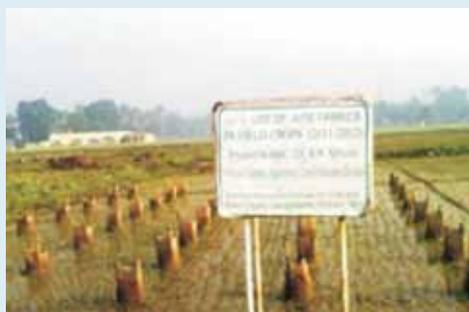
Jute reinforced soil columns in rice field
